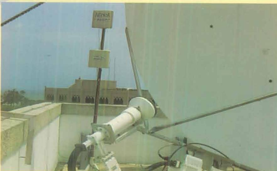
**Figure 6:** Two BWA antennas at 3.5 GHz can be clearly seen just close to receiver front
